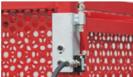
■ Safety valve that allows the operator to inflate the tire only when the door is closed.
