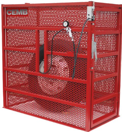
■ Its special structure consisting of iron bars and a beehive-shaped network makes the inflation cage TI-BOX extremely safe, because the pressure generated by any eventual tire explosion is contained by the cage and the leakage of fragments is extremely limited, thus reducing any damage to the operator.
