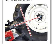
Tools holding arm and clamping chuck arm move in synch, keeping the tools perfectly tangent to the wheel, thus reducing tension and protecting rim and tyre from any damage.
